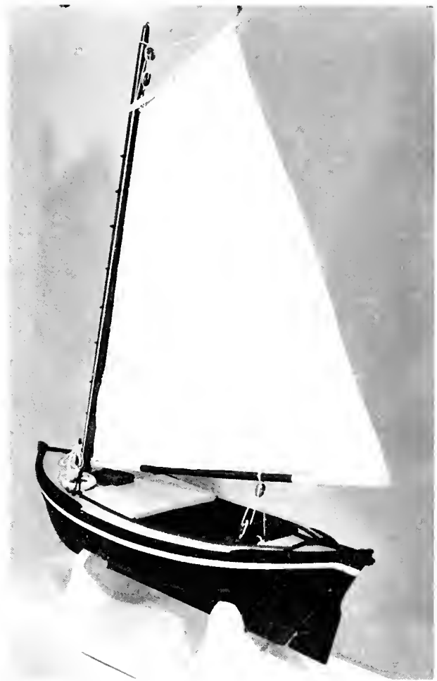
SARDINE CARRIER of the smaller size in use at Eastport, Maine, in the 1880's. This type was known as a quoddy boat, after Passamaquoddy Bay, Maine. Rigged model USNM 12099. (Smithsonian photo 45605-J.)
